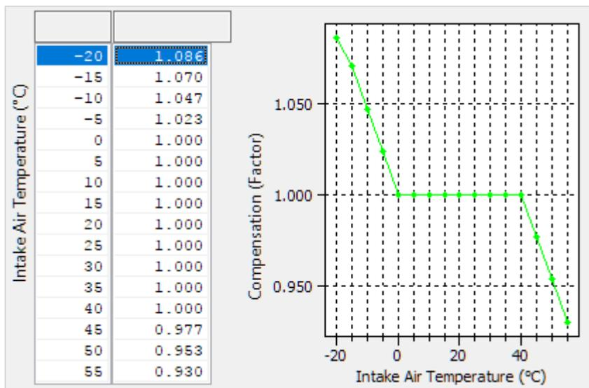
If the **SD Temperature Source** is set to *Use fixed calibration temperature* this map can be used to make adjustments to the calculated mass airflow based in *Intake Air Temperature*. It can be used in situations where SD is required on an otherwise standard car to deal with MAF limits, and a dedicated charge air temperature measurement solution is not in place.
