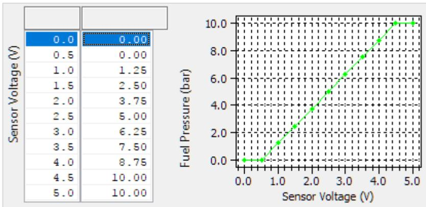
Sensor output based on input voltage.
