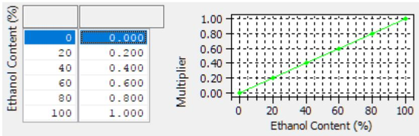
The boost limit for ethanol is blended in the same way as the boost target.
