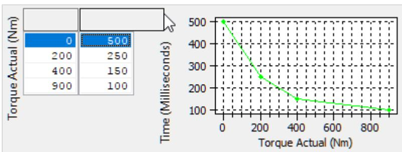
Clutch slip will be ignored for this amount of time after an increase in current gear. This is used to ignore normal levels of slip during and shortly after a gearshift.
