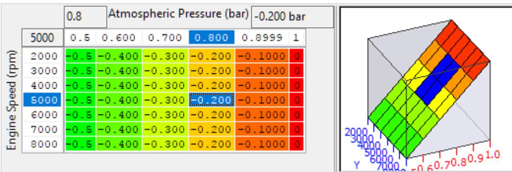
The boost target can be offset for changes in atmospheric pressure the default map values reduce the absolute boost target 0.1Bar for each 0.1Bar drop in atmospheric pressure. This is suitable for stock turbos which will often be pushed to their maximum at sea level, and pushing the same absolute pressure at altitude can be detrimental to the turbos while not giving the desired pressure.
