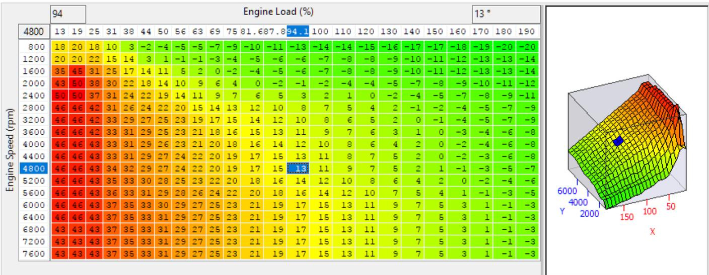
Four maps, one for each mapswitch mode providing an easy to understand and tune base ignition value in degrees BTDC. They provide increased precision and headroom for the load axis and increased RPM breakpoints. It's possible to create multiple maps and use map switching to cycle between each map for testing.
