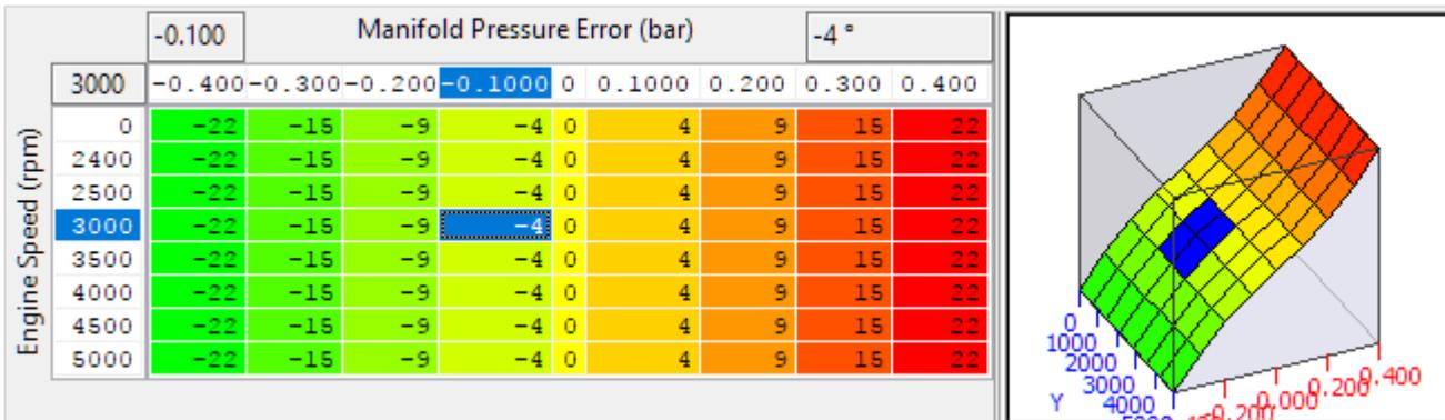
Used in conjunction with **Rolling Launch Ignition Timing Base** to deliver the **Rolling Launch Target Manifold Pressure** typically using increased retard to increase boost. The final ignition value will be capped at -30deg (30deg ATDC).
