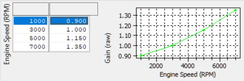
The level of torque reduction is dictated by the gain values in this map and the amount of unwanted clutch slip *Clutch Slip Error* which is defined as:
