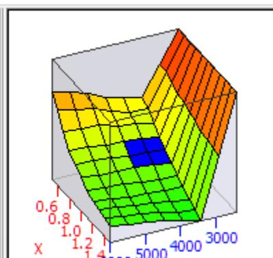
Sets the base timing while BOTL is active, instead of the main ignition map for each Mapswitch Mode. The ignition timing values are very low to promote making boost, but caution should be employed before lowering them too far as excessively retarded ignition timing will result in sluggish RPM control on launch and potentially boost that is too high and hard to control.
