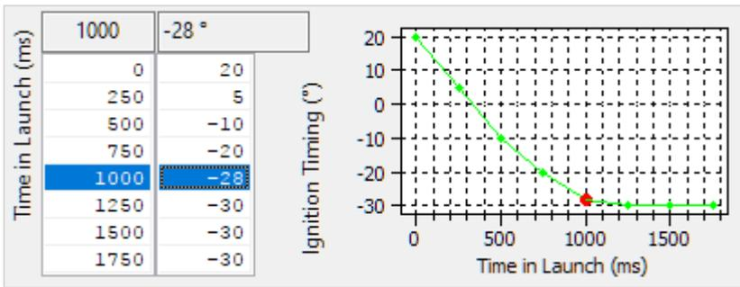
This prevents an instantaneous significant ignition timing change due to BOTL from causing a sudden drop in engine RPM and subsequent cycling of RPM and BOTL switching on/off.
