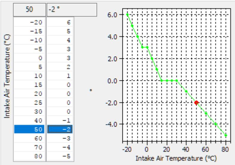
An ignition timing offset based on *Inlet Air Temperature* which can be used to retard the ignition for high air temps. This is particularly useful on cars modified to put the IAT sensor in the low temperature boost pipe (after intercooler) as retard can be applied for charge temperature directly.
