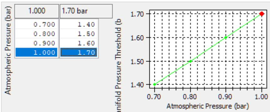
A threshold of manifold absolute pressure above which the integral correction is activated.
