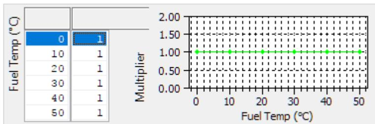
When tuning a car with a fuel temperature sensor, it is now possible to compensate for changes in the fuel temperature. Typically fuel pulsewidth is increased with increasing fuel temperature to compensate for the drop in fuel density, numbers greater than 1.0 will increase injector effective pulsewidth.
