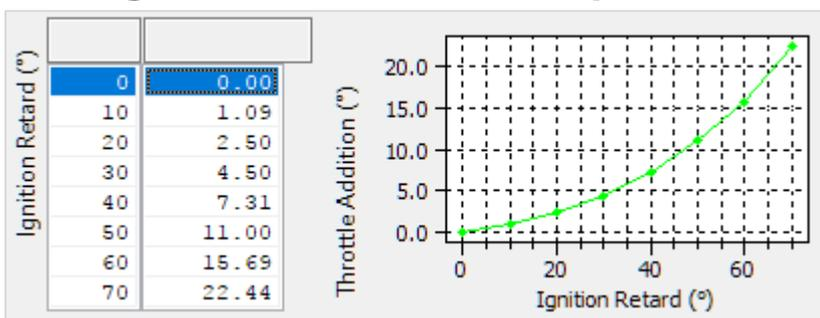
This map adjusts the throttles to compensate for torque variations as the ECU varies the ignition timing to generate boost. The compensation is now an absolute throttle angle adder and the above table has shown to give sensible results but may need fine tuning.
