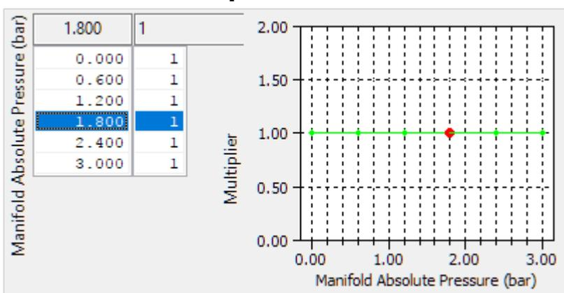
This can be used to multiply the fuel quantity while in launch control to make broad corrections for errors in AFR.
