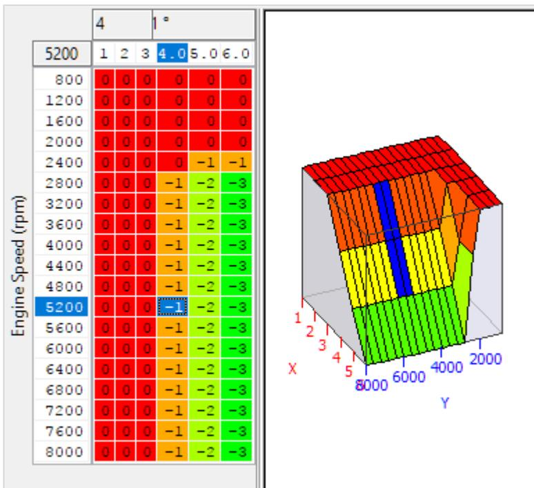
Ignition advance can be trimmed on a per gear basis, relative to RPM using this map. It would be normal to reduce advance in higher gears at high RPM or at an RPM sensitive to detonation.
