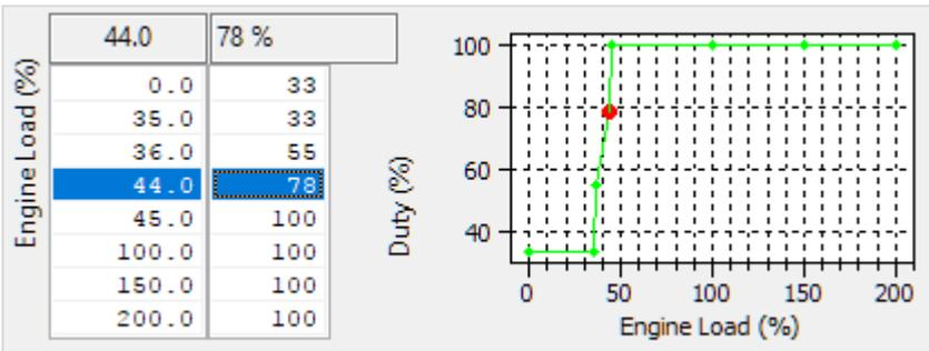
Direct fuel pump control is ONLY ENABLED WHEN 12 INJECTOR CONTROL IS ENABLED! So if you wish to use these maps, enable 12 injector control in all your map switch modes and set the enable RPM to 10000rpm so that it never comes on. Remember when 12 Injector Support is enabled the secondary air solenoid output will be hijacked.
