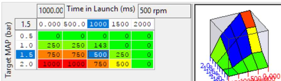
The overshoot RPM is added to the base RPM value to temporarily raise the RPM limit at the beginning of Launch Control to help the boost to be more quickly increased to the target level.
