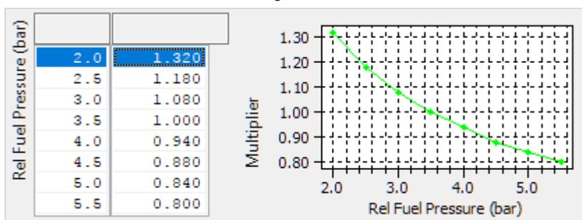
Changes in fuel pressure can be compensated for using this new map, in conjunction with an additional sensor configured using the new sensor options. For the purposes of this correction *Relative Fuel Pressure* is used and represents the pressure difference between the inlet (fuel rail) and nozzle (inlet port) pressures, defined as:
