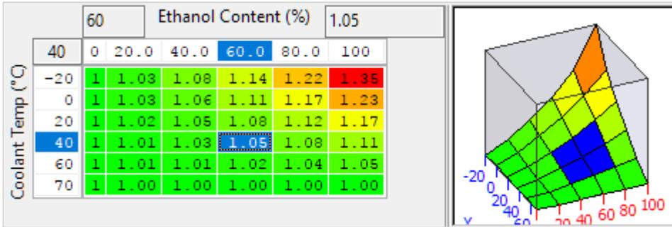
The fuel quantity at cranking will be affected by the **FlexFuel Quantity Multiplier** map however it may be required to change the fuelling further at low temperatures when cranking. This map is a 0-2 scalar and will multiply the base fuelling only when cranking.
