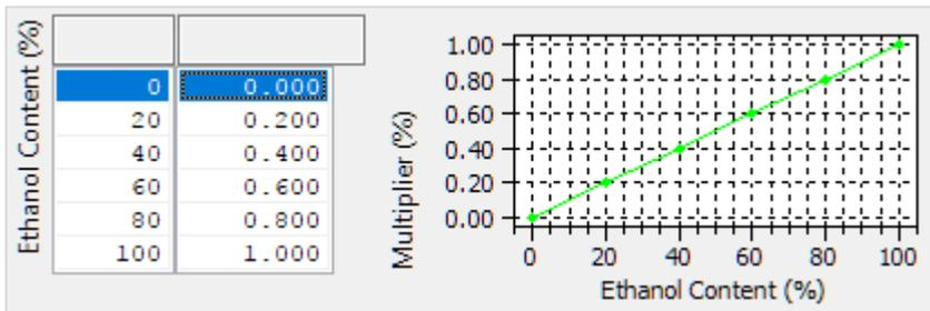
The values are a multiplier of the **FlexFuel Ignition Timing Max Addition** values and dictate how much of that advance is added for a given Ethanol content. The resulting ignition advance is calculated as ((Gasoline Ignition Timing + (Blend Multiplier \* FlexFuel Ignition Timing Addition)).
