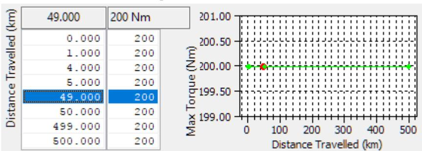
When Valet Mode is active the torque output can be limited to prevent a car being driven hard or recklessly. For use as an anti-theft measure it would be reasonable to reduce these values from the default 200Nm after a short distance.
