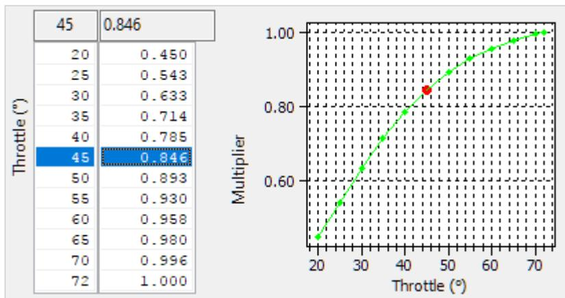
The boost target as adjusted by the **Boost Target Atmospheric Correction** map is multiplied by the output of this map. For example, a target of 2.4bar \* 0.45 = 1.08bar absolute.
