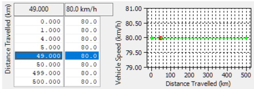
When Valet Mode is active the maximum speed can be limited to prevent the car from being driven at anything beyond a sedate pace. For use as an anti-theft measure it would be normal to significantly reduce these default values to as low as zero after a shorter distance.
