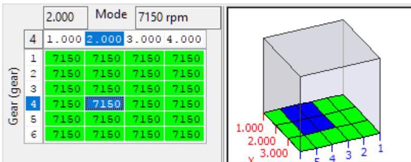
To simplify the setting of the fuel cut based rev limits, they now all appear in one 3d map and use a single 1d value to introduce hysteresis. The fuel cut will be active over the RPM value in this map, and fuel will only be restored when the RPM has dropped below this level by **Rev Limit Hysteresis**.
