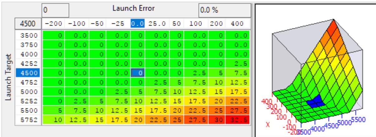
If BOTL ignition retard is active, this map also allows for a variable amount of fuel cut using the same cut strategy employed in custom maps, the resulting fuel cut percentage will be reflected in the *Cylinder Cut Probability* live data value. This can be used to help regulate engine speed, lower boost or just make a lot of noise.
