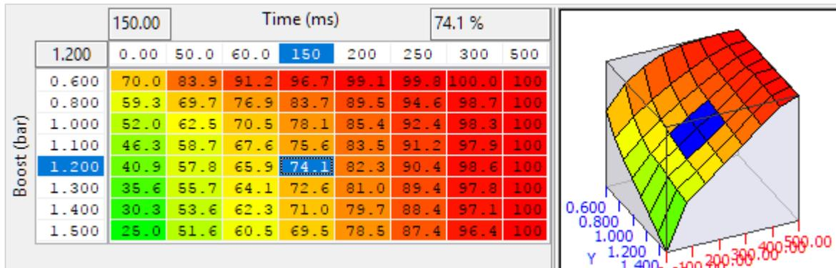
A temporary change in the Wastegate duty triggered with an upshift to prevent the boost spikes on gearshift caused by a sudden change in the air consumption of the engine as the RPM drops. The X axis is time since the start of an upshift, and the Y axis is the relative boost in Bar at the time the shift was triggered.
