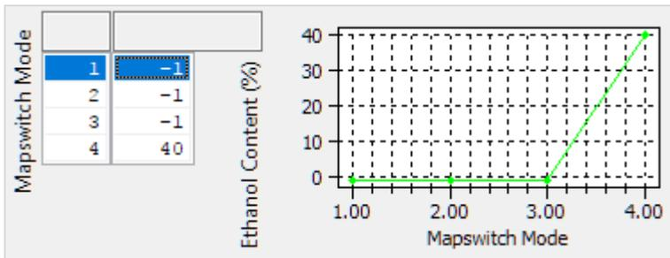
It is not always practical to add a FlexFuel sensor to every car that uses alcohol in the fuel, and many users may wish to pre-mix a specific amount of ethanol, methanol or E85 with their regular gasoline to improve performance. Pre-mixed ratios of alcohol can now be catered for in the RaceROM FlexFuel strategy but entering the ethanol content in this map.
