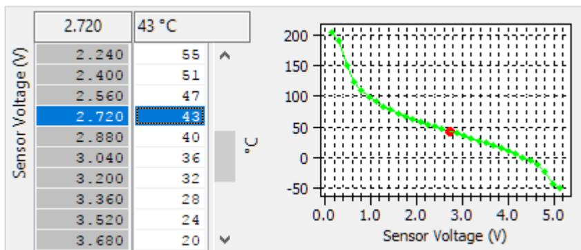
In the stock implementation, the Intake Air Temperature sensor shares its scaling data with the engine coolant temperature. If replacing the IAT sensor, it's possible to use the RaceROM scaling instead to cater for non-standard scaling without disrupting the ECT sensor scaling. Use of this scaling map is enabled in **Speed Density»SD Enable**.
