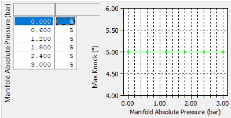
A threshold of the maximum level of knock retard that is permitted before limp mode is triggered. The values in the map equate to retard, so a limit of 5 will be triggered when *Knock Correction* reaches -5 degrees.
