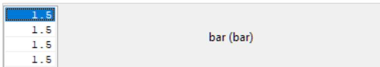
The base target Manifold Absolute Pressure while the Rolling Launch anti lag is active. This target is capped by the limits set in **Rolling launch Maximum Boost Target** and the result is used as the target for the ignition retard maps as part of the antilag system.
