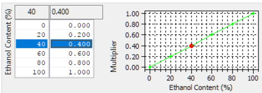
This map combines **Boost Target by Gear** and **FlexFuel Boost Target by Gear** to derive the final boost target based on *FlexFuel Ethanol content*. The eventual boost target is calculated as:
