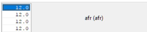
AFR target override to be used while the Rolling Launch retard is active, this should be set reasonably rich to help keep exhaust temperatures from become extreme.
