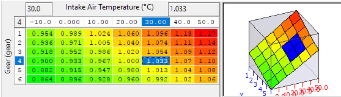
The output of the Wastegate base duty map can be multiplied to increase or decrease it to compensate for changes in intake air temp and/or gear. Typically the base duty is increased with values greater than 1.0 for lower gears (1<sup>st</sup>/2<sup>nd</sup>) to improve spoolup with rapidly changing RPM. Conversely the base duty is often decreased with values of less than 1.0 for higher gears (5<sup>th</sup>/6<sup>th</sup>) to prevent overboost with increasing load and slower RPM rates.
