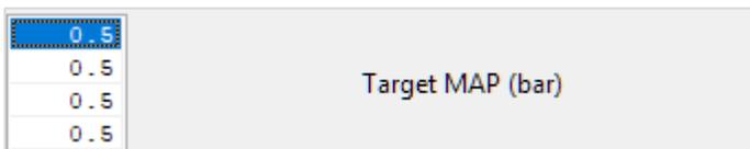
Using EcuTek's iPhone and Android companion App - ECU Connect, the BOTL target boost can be altered between limits set for each Mapswitch Mode. By default, both the min and max limit are set to the same default values for **LC MAP Target** and will require calibration to allow manipulation from within ECU Connect.
