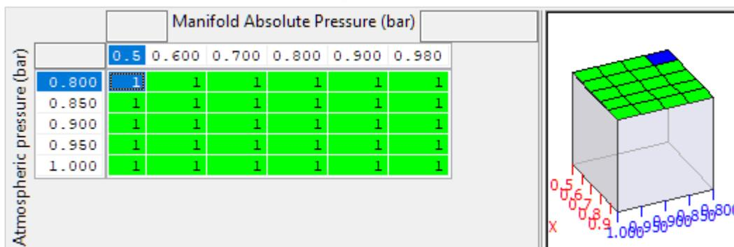
This can be used to compensate for the changes in VE typically experienced at high altitude and low atmospheric pressure. The values will multiply the VE from the SD VE map.
