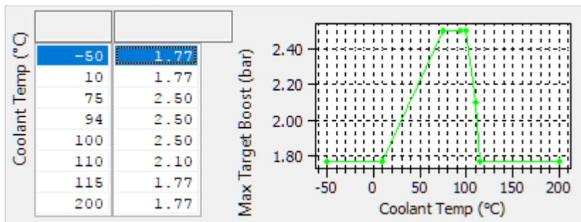
Maximum target based on engine coolant temperature, used as a maximum limit for boost target at normal engine temps and reduced significantly at excessive temps for engine safety.
