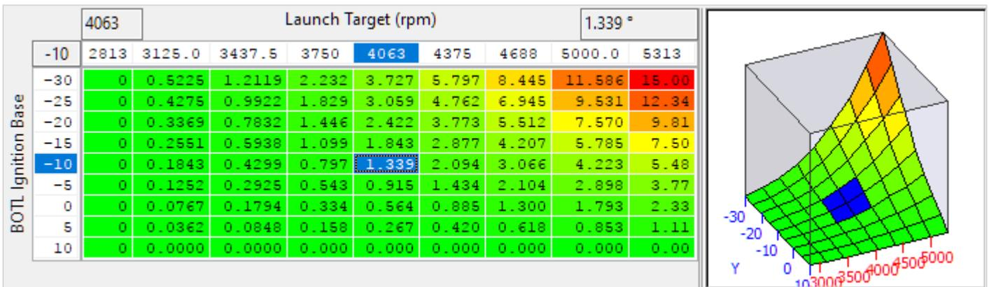
This adds an offset to the normal throttle angle depending on the current BOTL ignition retard, which is defined as the difference between the normal ignition timing as determined by the RaceROM Ignition Map for the current Mapswitch mode, and the current actual ignition timing as set by the BOTL strategy.
