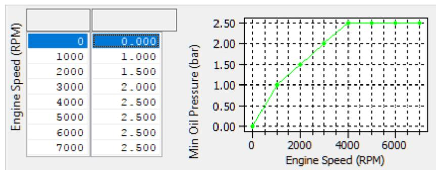
When using a RaceROM equipped ROM in the TCM the ECU can receive oil pressure information and use this for checking for issues. To trip the oil pressure limp mode, the measured pressure needs to drop below **Oil Pressure Minimum** for at least **Oil Pressure Timeout**.
