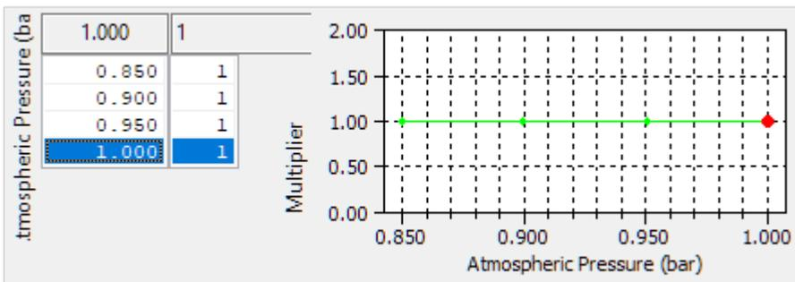
This map defines how the high and low altitude base maps are combined to produce the wastegate base duty. A value of 1.0 uses only the value from the low altitude (sealevel) base map, a value of 0.0 uses only the value from the high altitude base map. The final value for *WG Duty Base* is calculated as:
