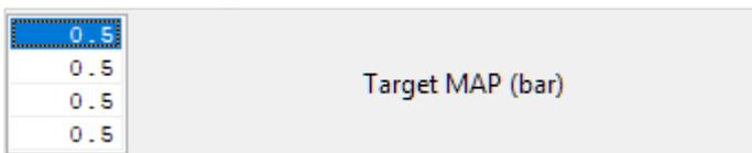
A target of Manifold Absolute Pressure to achieve using the Boost Off The Line strategy, the default values of 0.5 represent 0.5bar absolute, in other words 0.5 bar of vacuum (at near sea level).
