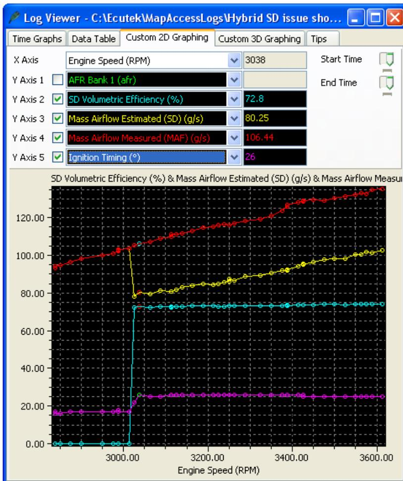
This is **BAD** hybrid tuning and the car even had clutch slip problems during transition. In this example the SD is switched ON at 3000rpm.
