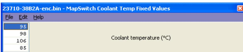
So when MODE 1 is selected the Coolant Temp gauge will show 95 (**203F**)
