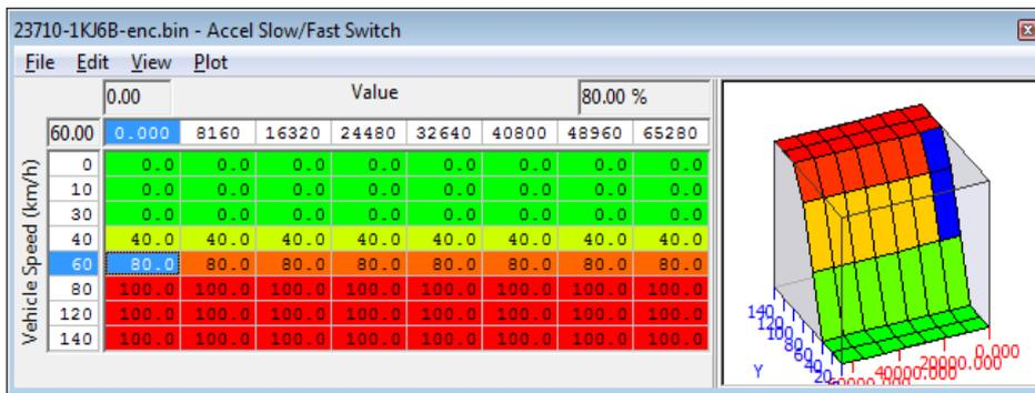
Alternate maps are used whilst in Safe Mode from the regular Normal Mode maps.
