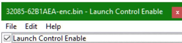
Overall enable for the launch control strategy enabled when box is checked, enabled by default on later ROMs.
