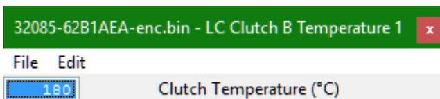
Maximum clutch B temperature allow at launch. LC will not activate if the temperature already exceeds this value.
