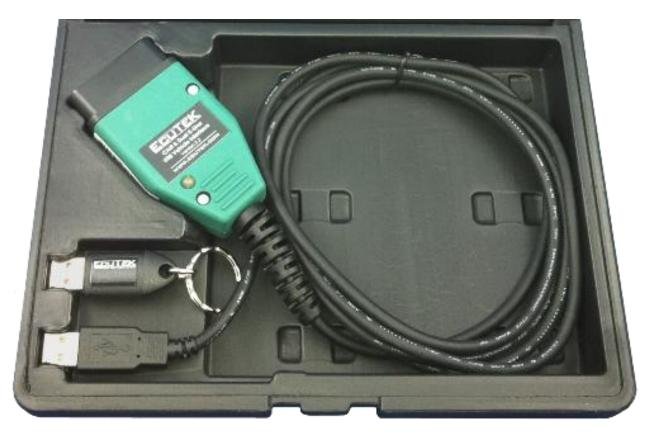
The programming interface plugs into the diagnostic port of the car, and allows communication with the ECU.
