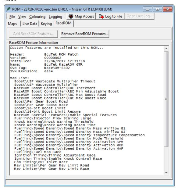
When the Feature File is applied, data is automatically copied from the existing ECU maps into the new maps that are being created. This preserves any tuning work that has already been done to the ROM.
