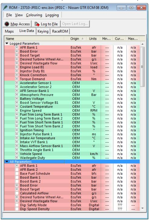
All the items marked as **EcuTek** in the Origin column are RaceROM custom data logging parameters.
