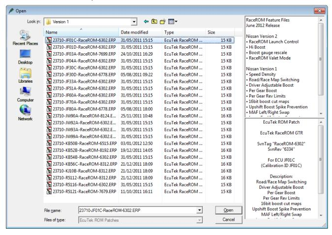
IMPORTANT: The Feature File must have EXACTLY the same name as the ROM file. For example: It is NOT possible to apply a JF01D Feature File to a JF01C ROM.
