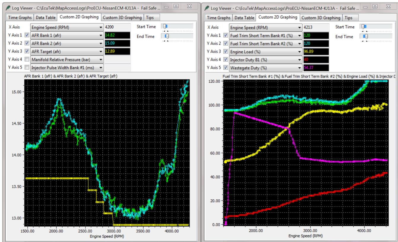
The left hand side shows the AFR becomes lean at higher RPM due to lack of fuel delivery. The right hand side shows the FTST climbing to 120% trying to add more fuel but the AFR is climbing out of control and is dangerously lean at 15:1. The engine will be seriously damaged!
