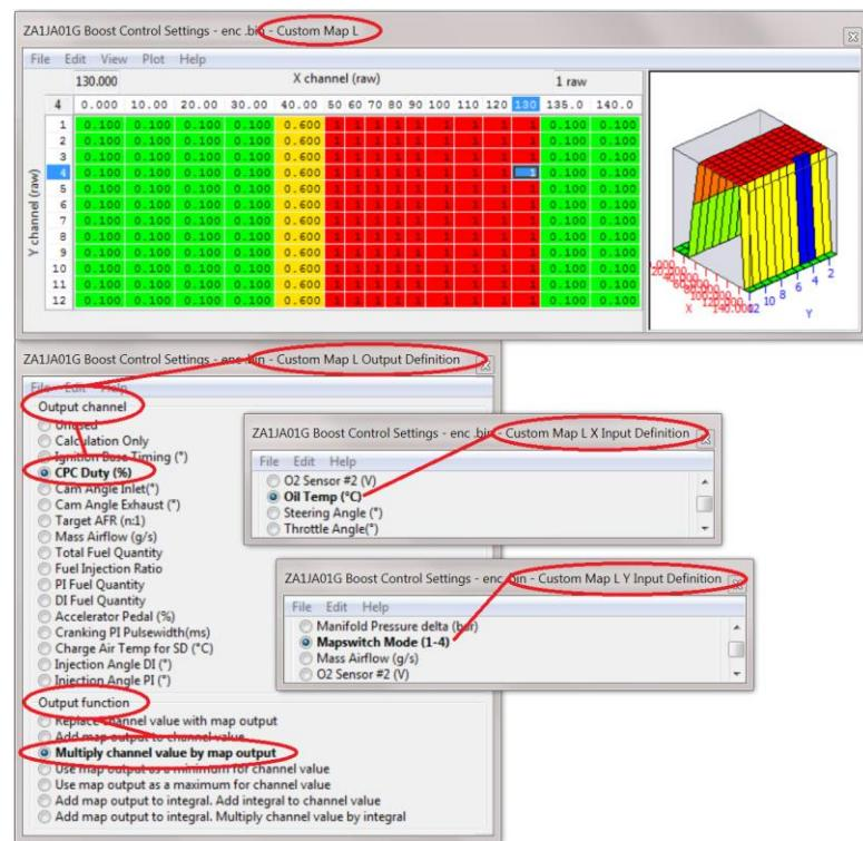
Custom Map L below has been configured to multiply the WG Duty dependant on the current Oil Temp (X axis) and the current Map Switch mode selected (Y axis).
