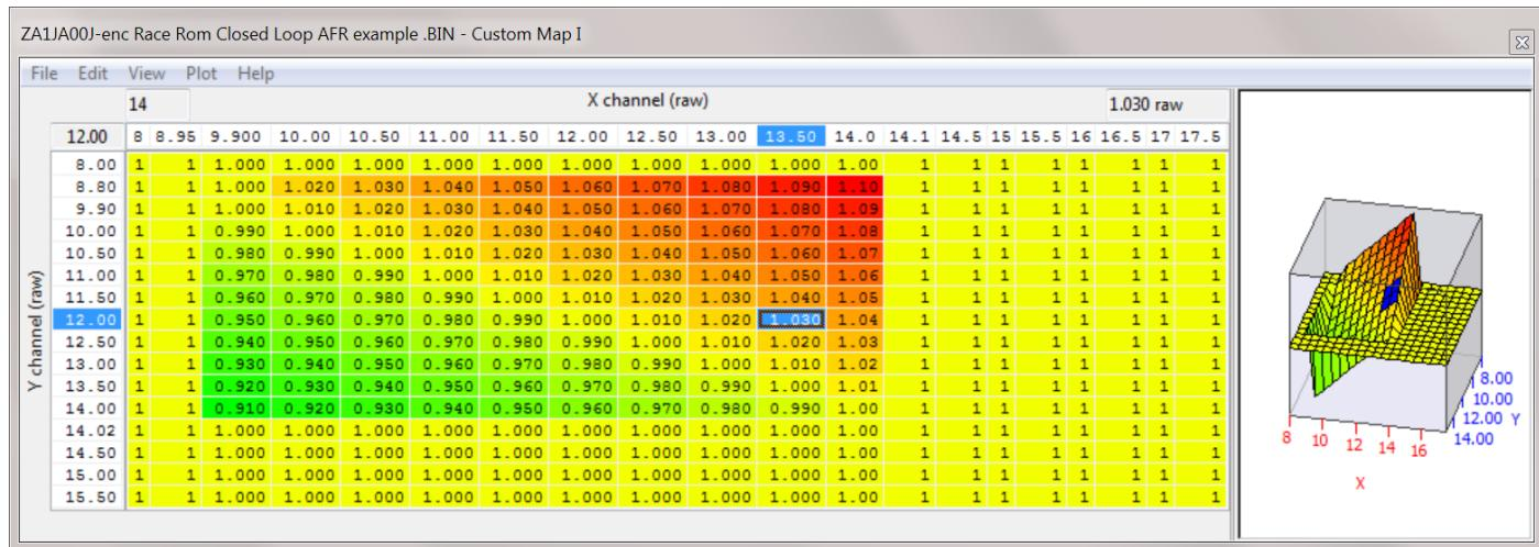
The compensation could be an Integral addition/subtraction for a proper closed loop control (though you would want to set a min and max for the Integral amount). We would suggest an Integral Min/Max of 20%.
