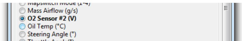
When logging this value be sure to use the EcuTek "O2 Sensor #2 – Voltage" parameter, because the OEM parameter of the same name displays a maximum of 1.275volts, even when the actual voltage is higher.
