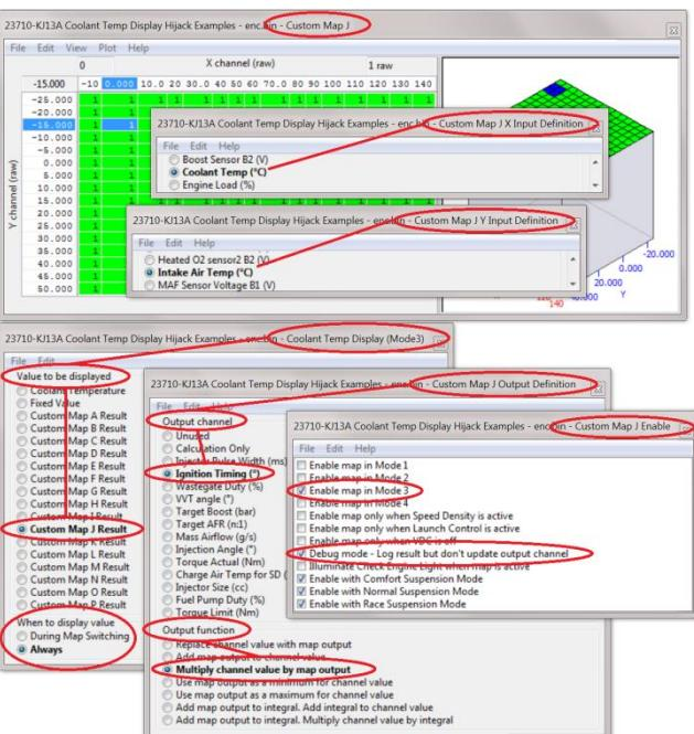
The important thing to note here is there is no Ignition Timing input definition parameter.
