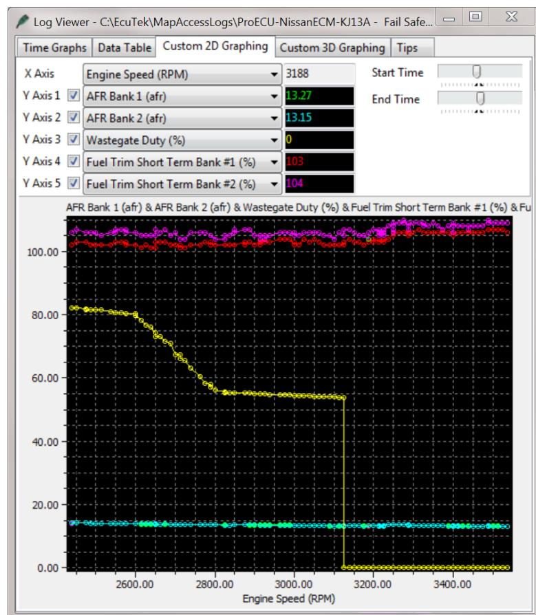
Now see the same 2<sup>nd</sup> fuel pump failure event again when the Fail Safe Custom Map G has been enabled.
