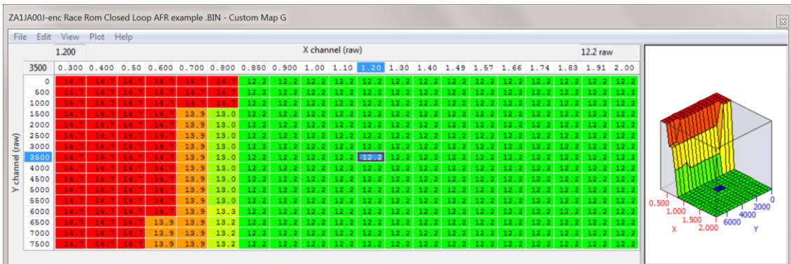
So when the Wideband AFR reading is leaner than the Target AFR then the fuel volume amount would be increased.
