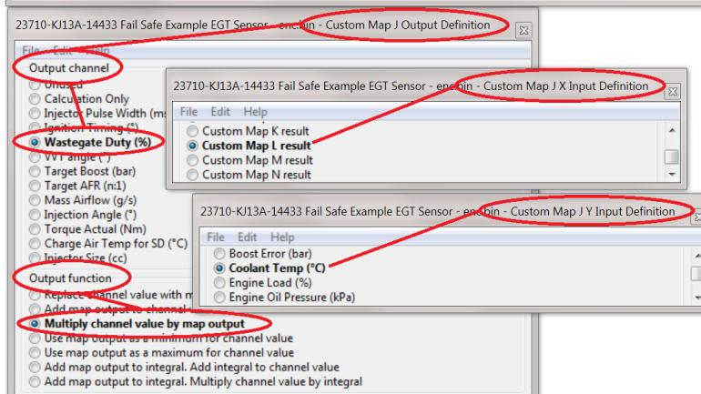
The output of Map L will be **Calculation Only**; it is now imported into **Custom Map J** which will reduce WG Duty for the highest EGT reading and Coolant temp.
