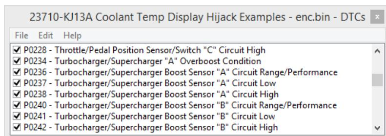
When using Boost Sensor #1 or #2 for Fuel Pressure or Charge Air then be sure to disable DTCs P0236 or the voltage will not read correctly, NOTE that this DTC does not illuminate a CEL and the channel will not update in Custom Maps if this DTC is not disabled.
