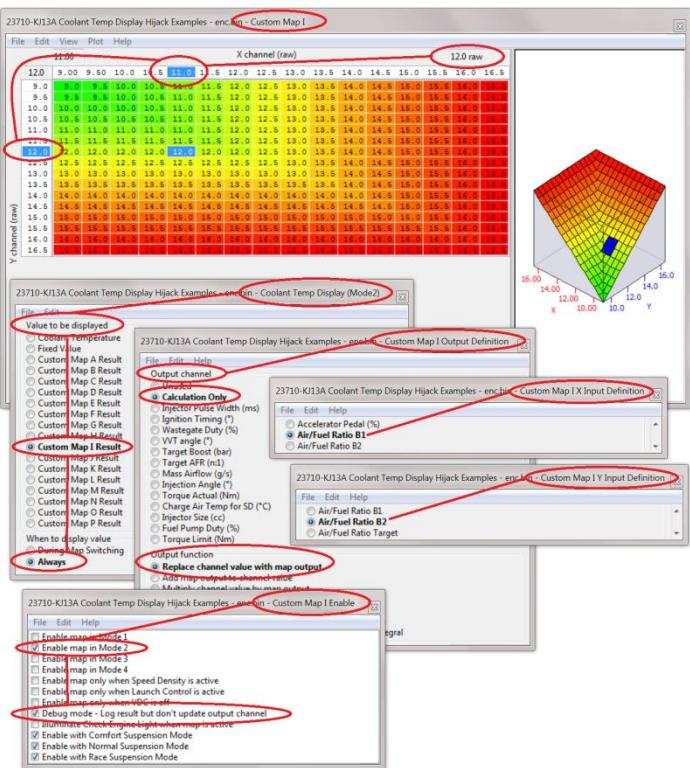
Custom Map I will output the leanest AFR from B1 or B2. The result of Custom Map I will be displayed on the Coolant Temp Display in Mode 2 **Always** (and not just during **Map Switching**).
