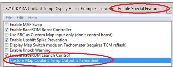
On the latest RaceROM Feature Files (RRFF) there is an option for US region vehicles to show the correct value found under Enable Special Features section.
