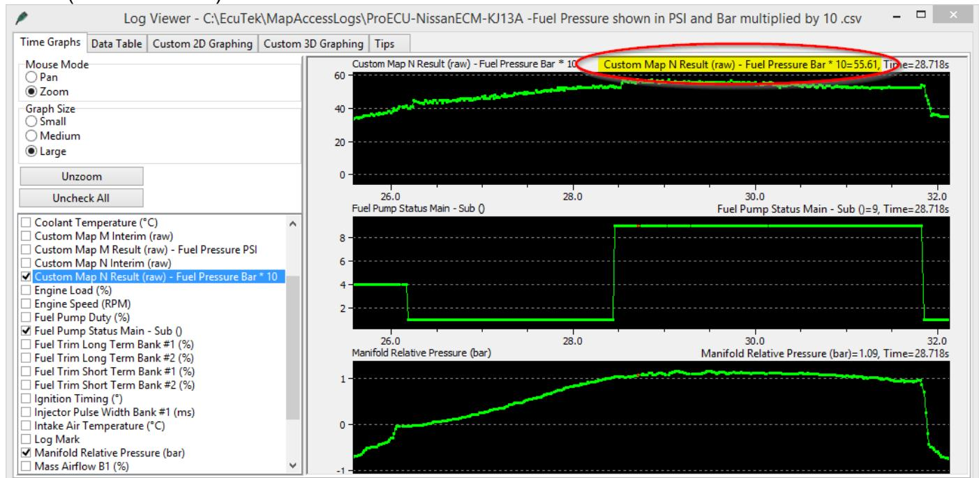
Remember that for US region models show Coolant Temp as Fahrenheit instead of Centigrade the Enable Special Features check box for Fahrenheit should be selected so the Fuel Pressure is shown correctly.
