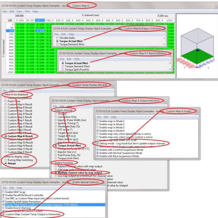
The result of Custom Map K will be displayed on the Coolant Temp Display in Mode 4 **Always** (and not just during **Map Switching**).
