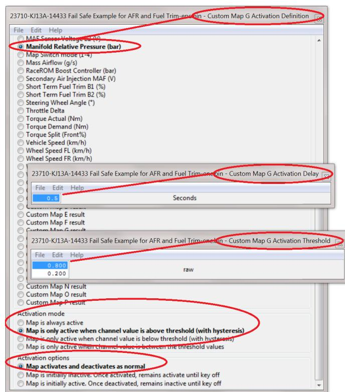
We should also set up a load based activation threshold for this fail safe to be allowed to work.
