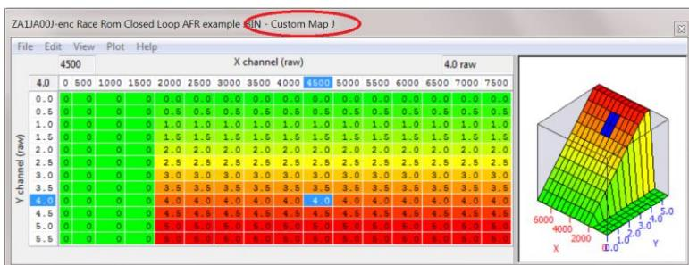
The X axis is RPM and the Y axis is CPC Sensor Input for the 5v potentiometer.
