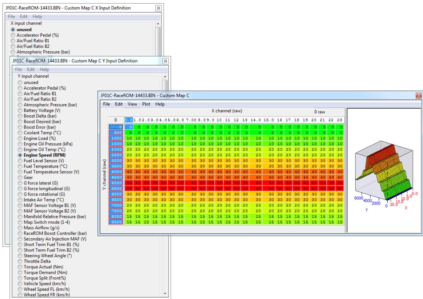
The X input channel is "unused", therefore the X input value will always be zero. Only the zero column on the map will be used, but it is very important to provide a complete X axis in ascending order. Otherwise the ECU's map lookup function may not work correctly. Always make sure to fully populate the maps and their axes with sensible values.
