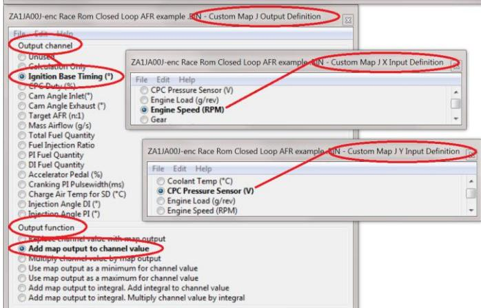
This Cosworth BRZ project development testing shows the Injection Firing Angle and Ignition Timing being adjusted simultaneously with two potentiometer voltage inputs, on the GTR there are 7 voltage inputs to play with.
