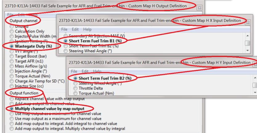
**NOTE:** It's important to notice the X and Y axis where there is a defined step between 119% and 120% so the WG Duty is either ON or OFF.
