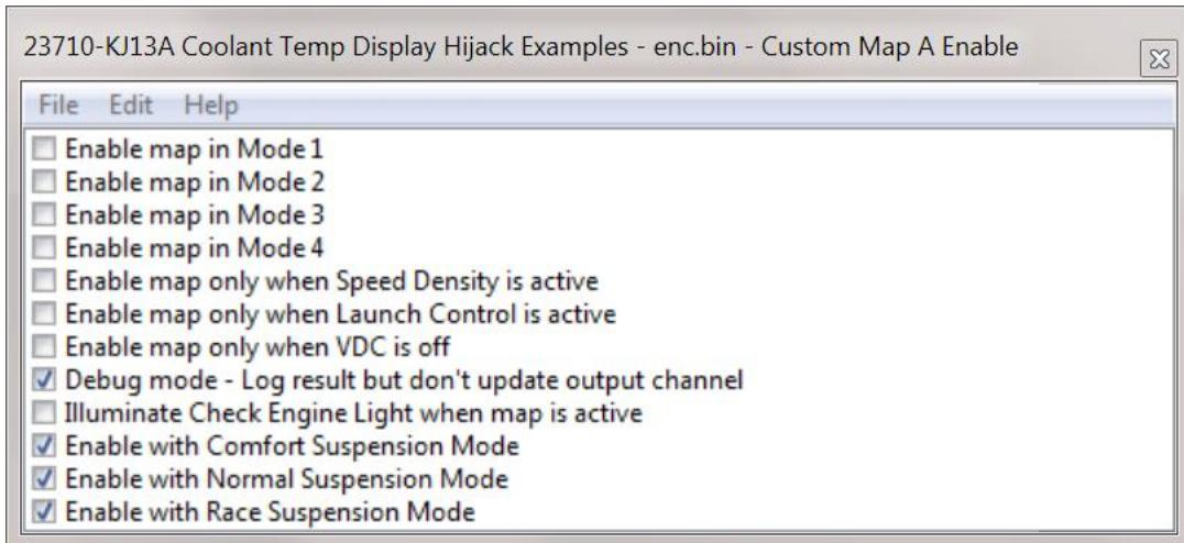
When used in conjunction with our Phase 4 TCM upgrade or newer, custom maps can be enabled depending on the position of the suspension mode switch. You must have at least **one** of the suspension mode checkboxes selected in order for the map to be active. By default, maps are active in all three modes.
