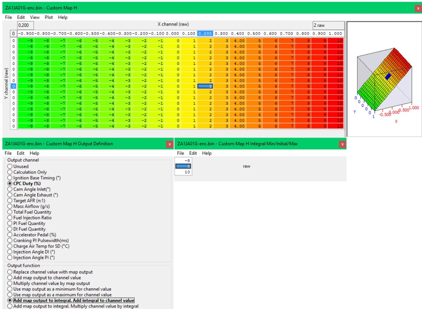
For the purpose of illustration, assume the map result is always 2. The first time the map is processed, the map result is 2, and this gets added to the integral  $0 + 2 = 2$ . Then the integral gets added to the output channel (CPC Duty which is used for Wastegate Duty on BRZ). So the final calculation is (CPC Duty + 2).
