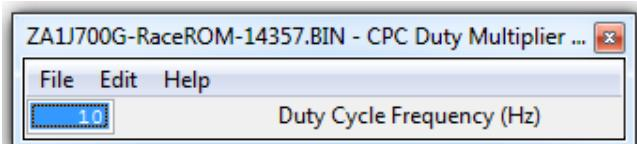
The frequency of the solenoid should be adjusted by the "CPC Duty Multiplier" map in order to obtain the best result for your application. Most WG Duty solenoids work best around 30% to 35% Hz.
