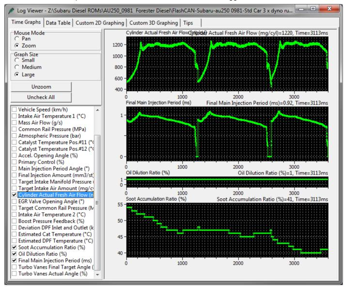
The **Soot Accumulation Ratio** parameter can, for example, indicate if the **Force DPF Regeneration** tool should be used. If the Soot Accumulation exceeds 65% then an Active Regeneration (Regen) will commence when conditions are correct (engine up to temperature, driving over 50kph for 10 minutes etc)
